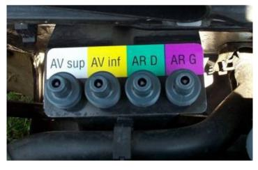
Connector AR G (Rear block left hand side) Connector AR D (Rear block right hand side) Connector AV inf (Front lower block) Connector AV sup (Front upper block)
